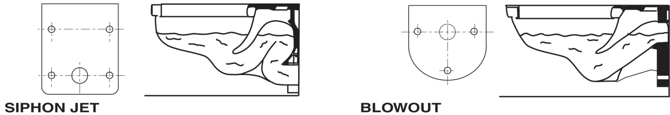
Figure 3. Water Closets: Types and Support Structures.
