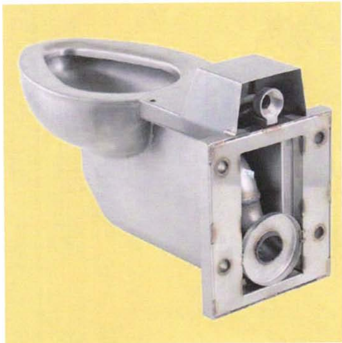
> Figure 4. Back view of an elongated bariatric-duty wall-mounted toilet bowl – rated up to 1,000 pounds.
