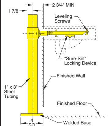
**SUFFIX -M31 Rectangular Steel Uprights with Welded Bases.** For use with metal stud and sheet rock wall construction. The rectangular shape upright offers greater structural strength and does not rely on the wall construction for support of the fixture. The rectangular upright keeps deflection to a minimum. For use with all floor mounted fixture supports. Add Suffix -M31 to figure number required.
