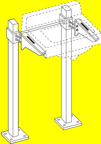
Vitreous China lavatory designed for use with acid resistant coated exposed arm support. Specify Fig. 0870 (-M31).
