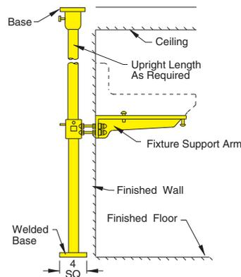
**SUFFIX -M11 Floor-to-Ceiling Uprights** When required, floor mounted fixture supports can be supplied with floor-to-ceiling uprights for securing to the floor and to the ceiling above. Add Suffix -M11 to figure number required.
