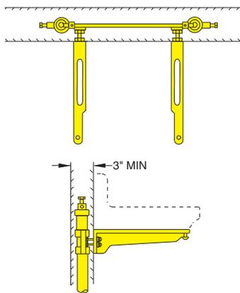
**SUFFIX -Z Special Narrow Sleeve and Base for Exposed Arm Support.** When an exposed arm lavatory or sink support is to be installed in a narrow wall, a special narrow sleeve and base are available for this type of installation. Add Suffix -Z to figure number required.
