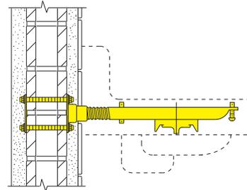
**WALL MOUNTED SUPPORT** - The function of this support is to provide for securing of the fixture to the wall in areas where a floor mounted support cannot be installed. The wall structure must be of sufficient strength to support the entire weight of the fixture.
