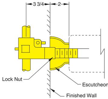
**SUFFIX -E Threaded Escutcheon.** When using lavatories of the flat slab type, the manufacturer requires a 2" dimension from the face of the wall to the rear of the lavatory. The 2" dimension prevents water from accumulating at the wall and causing deterioration. The escutcheon is chrome plated and is available on all concealed arm type supports. Add Suffix -E to figure number required.
