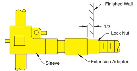
**SUFFIX -M24 Extension Adaptor for Concealed Arm Support.** When the standard (3 3/4") dimension from the face of the wall to the centerline of support upright, as shown in the illustration, is exceeded, use Suffix -M24 extension adaptor. The face of the extension adaptor should be set 1/2" in back of finished wall so the standard concealed arm and locking arrangement can be used for the lavatory regardless of the wall thickness. Add Suffix -M24 to Fig. No. required.
