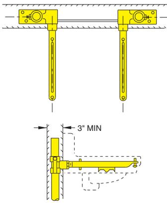
**SUFFIX -Z Special Narrow Sleeve and Base for Concealed Arm Support.** When a concealed arm lavatory support is to be installed in a narrow wall, a special narrow concealed arm sleeve and base are available for this type of installation. Add Suffix -Z to figure number required.
