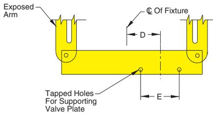
**SUFFIX -KF Supporting Bar for Fixture Mounted Knee-Action Valve.** Can be furnished on any exposed arm, wall or floor mounted sink support. Add Suffix -KF to figure number required.
