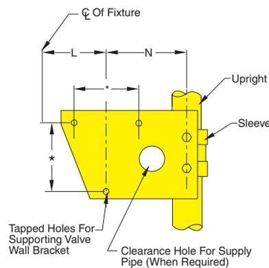
**SUFFIX -KW Supporting Plate for Wall Mounted Knee-Action Valve.** Can be furnished on any floor mounted lavatory or sink support. Add Suffix -KW to figure number required.
