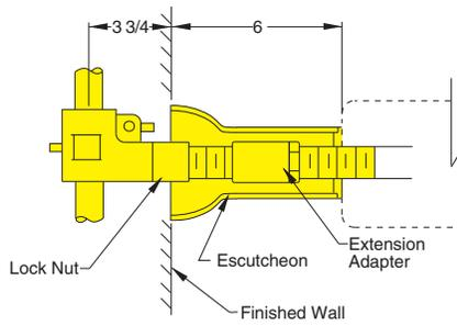
**SUFFIX -E6 6" Long Threaded Escutcheon.** When lavatories of the flat slab type are to be set away from the wall beyond the normal 2" setting, a 6" long escutcheon is provided with the same threaded arrangement as the regular 2" escutcheon. This escutcheon is chrome plated and is available on all concealed arm type supports. Add Suffix -E6 to figure number required.
