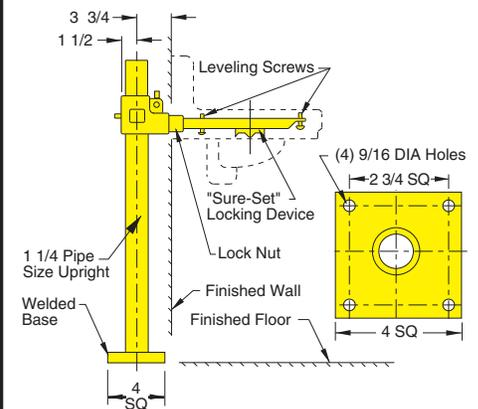
**WELDED BASE Regularly Furnished.** Round steel upright with welded base. Used with floor mounted fixture supports. The base should be securely anchored to the floor construction w/(4) 1/2" bolts. (By others)
