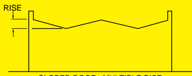
SLOPED ROOF - MULTIPLE RISE
