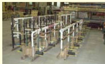
Fig. No. 0210RY-M54, 0210DY-M54 and 0710. Angle iron Pre-Fab with PVC piping.
